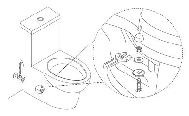
\*\*NOTE: Do not overtighten nuts. Porcelain is fragile and could possibly crack if nuts are overtightened.\*\*
